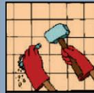
**Tip: Inspect your shower** for crack or missing grout between tiles. Repair missing caulk or grout. Reseal tile with masonry sealer, which can be purchased at most paint or home improve-
